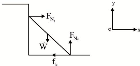
$$\begin{cases} F_{net_x} = 0 \rightarrow f_k = F_{N1} = 100\text{ N} \\ F_{net_y} = 0 \rightarrow F_{Nr} = W = 240\text{ N} \end{cases} \rightarrow R = \sqrt{f_k^2 + F_{Nr}^2} \rightarrow R = \sqrt{100^2 + 240^2} = 260\text{ N}$$
