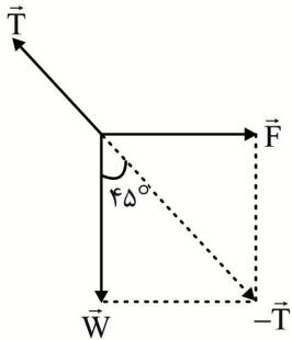
$$\tan 45^\circ = \frac{F}{W} \rightarrow F = W \rightarrow \frac{kq^r}{r^2} = mg \rightarrow r^2 = \frac{9 \times 10^9 \times 4 \times 10^{-18}}{40 \times 10^{-9} \times 10} \rightarrow r^2 = 0/09 \rightarrow r = 0/3m$$
