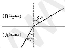
$$\frac{\sin \theta_A}{\sin \theta_B} = \frac{n_B}{n_A} = \frac{v_A}{v_B} = \frac{\lambda_A}{\lambda_B} \rightarrow \frac{\sin 30^\circ}{\sin 60^\circ} = \frac{\lambda_A}{\lambda_B}$$
