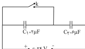
$$C_{eq} = \frac{C_1 C_2}{C_1 + C_2} = \frac{6 \times 2}{8} = \frac{3}{2} \mu\text{F}$$
